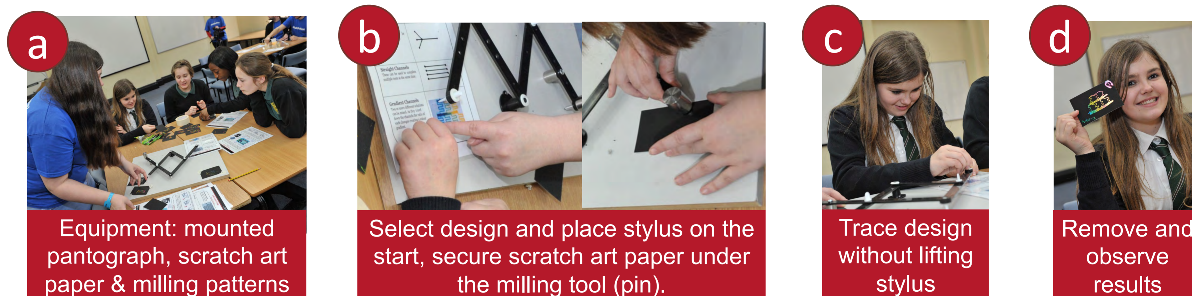
Fig. 2: (a) A pantograph (Sketch-a-Graph, purchased from Amazon) was secured to a base plate with a weight and a pin for 'milling'. (b) A design is chosen and scratch art paper (Baker Ross Scratch Art Doodle Sheets) is secured in place with Blue Tac. (c) The chosen channel design is traced. (d) Results are observed.
