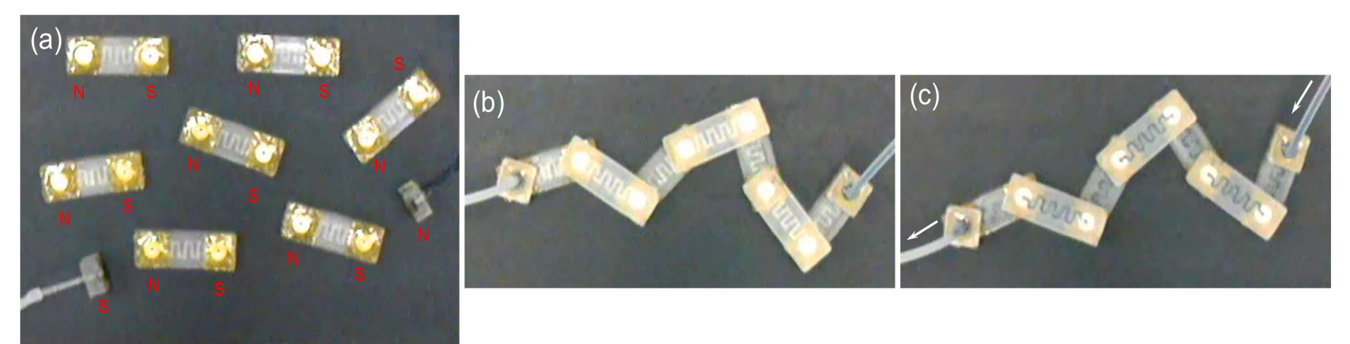
FIG. 3 7-serpentine channel modular microfluidic system using seven serpentine channel modules and two inlet/outlet modules. N and S represent the north and the south poles of the ring magnets, respectively. Kapton polyimide adhesive tape was used as the sealing gasket. (a) Before and (b) after assembly of the modular microfluidic system. (c) Assembled modular microfluidic system was filled with a blue colored food dye solution. The white arrows indicate the fluid flow direction and the fluid flow rate was 100 μl/min.
